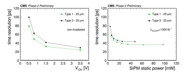
**Figure 5:** Comparison of the time resolution achieved with type 1 and type 3 modules. A better time resolution with thicker modules is achieved both with non-irradiated (left) and irradiated SiPMs (right).
