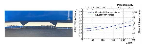
**Figure 3:** Left: Different LYSO array types (from left to right: type 1, type 2 and type 3). Right: BTL slant thickness along detector axis z.
