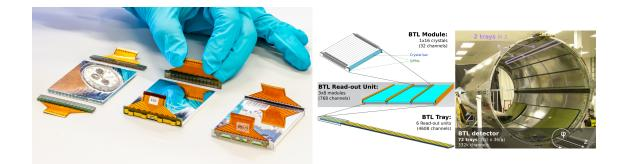
**Figure 2:** Left: Picture of BTL sensor modules. Right: Hierarchical structure of the BTL components (left) and trays enclosed within the mechanical support (right).
