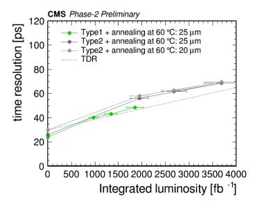
**Figure 6:** Time resolution as a function of the equivalent integrated luminosity (operation at T = -45°C and SiPM annealing at T = 60°C). Data are from test beam measurements of modules (both type 1, in green, and type 2, in grey) with non-irradiated and irradiated SiPMs and tested at various operating temperatures to emulate different points of detector lifetime.
