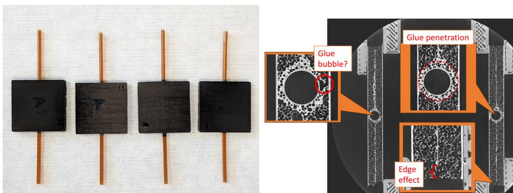
**Figure 4:** L: Prototype carbon-foam substrates R: X-ray tomography of substrate samples ((pictures courtesy of U. Manchester).
