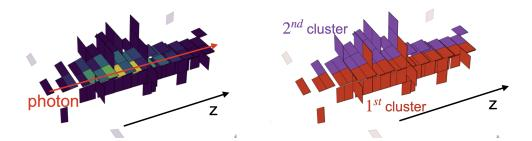
**Figure 3:** Cluster splitting in a simulated unconverted photon event in the HGCAL, produced using a 0 pileup sample. TCs coloured based on the energy (left), and on the cluster seed index (right).
