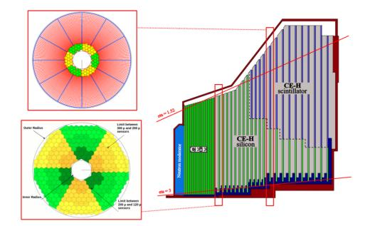
**Figure 1:** Schematic view of one HGCAL endcap slice (right), a mixed silicon and scintillators layer (top left), and a full silicon layer (bottom left). The majority of the HGCAL will be based on hexagonal silicon sensors with approximately  $1 \text{ cm}^2$  or  $0.5 \text{ cm}^2$  hexagonal cell sizes. The final HCAL interaction lengths in the low  $\eta$  region will be based on plastic scintillator with SiPM readout.
