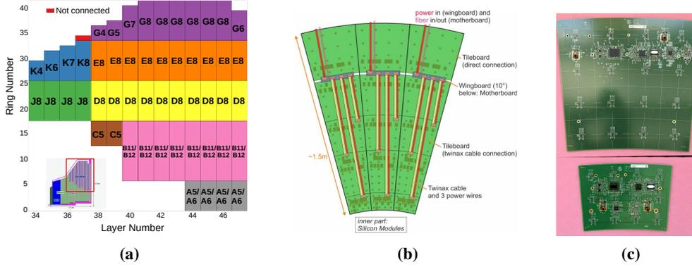
**Figure 2:** (a) shows the base layout of tile module geometry in a  $10^\circ$  sector to be used in the HGCAL. The letter symbolises the tile module type, and the number refers to the number of rings in the tile module. (b) shows the top view of a  $30^\circ$  sector showing only the scintillator tile modules [6]. (c) shows the largest tile module (G8) (top) and the smallest tile modules (A5) (bottom) placed next to each other.
