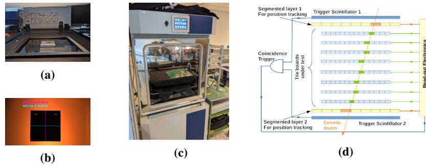
**Figure 5:** Three setups used for the quality control is shown here. (a) shows the scanning setup used at DESY to measure the tile sizes after wrapping in foil with one exemplary tile scan shown in (b) [12]. (c) shows a climate chamber at DESY which will be used for the thermal cycling of the PCB and fully equipped tile modules. (d) shows the sketch of a (conceptual) cosmic test stand for tile modules to be used at DESY.
