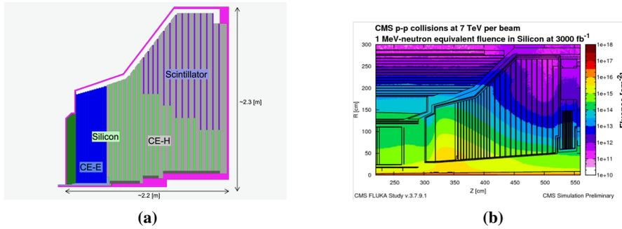
**Figure 1:** (a) shows a schematic view of the CMS high granularity end-cap calorimeter [4]. (b) shows the expected 1 MeV equivalent neutron fluence in silicon obtained from FLUKA studies at the end-of-life [1].
