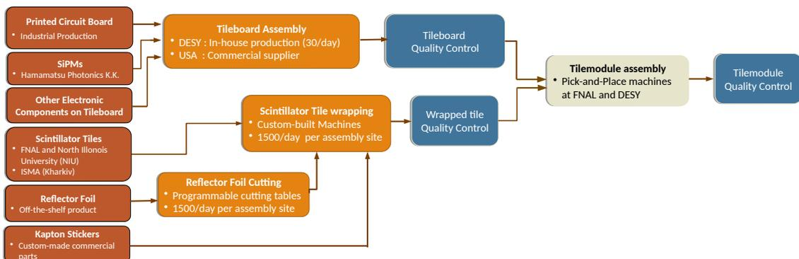
**Figure 3:** CMS HGCAL tile module production workflow [9]. tile modules before scintillators are installed are typically called as Tileboards.
