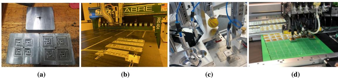
**Figure 4:** Four systems used in the production and assembly line. (a) shows the moulds used for the production of polystyrene-based injection-moulded scintillator tiles at FNAL [11]. (b) shows the machine at FNAL which will be used to cut the PVT-based tiles into shape [11]. (c) shows the tile wrapping station at DESY. (d) shows the pick-and-place machine used at DESY.
