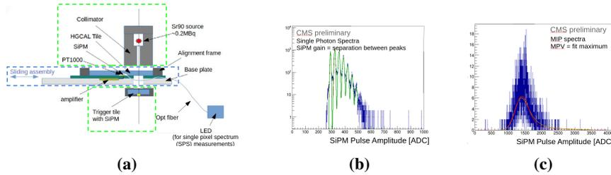
**Figure 7:** (a) shows the Strontium-90-based setup for scintillator quality control at DESY and CERN [14]. (b) shows a single-photon spectra from the SiPM and (c) shows a MIP peak obtained from a Scintillator under test.
