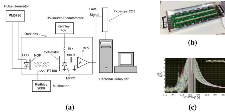
**Figure 6:** (a) shows a schematic of the SiPM quality control setup at CERN [13]. (b) is an array of SiPMs tested with this system. (c) shows the breakdown voltages measured.
