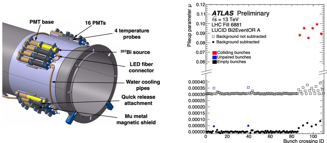
**Figure 1:** *Left:* Drawing of the LUCID-2 detector [5]. *Right:* Run averaged pileup parameter  $\mu$  as a function of the bunch-crossing identifier (BCID) as measured by the LUCID Bi2EventOR A algorithm. The empty squares (full circles) refer to the data before (after)  $^{207}\text{Bi}$  background subtraction. The red markers refer to the colliding bunch slots, the blue ones to unpaired-bunch slots, and the black ones to nominally empty slots [7].
