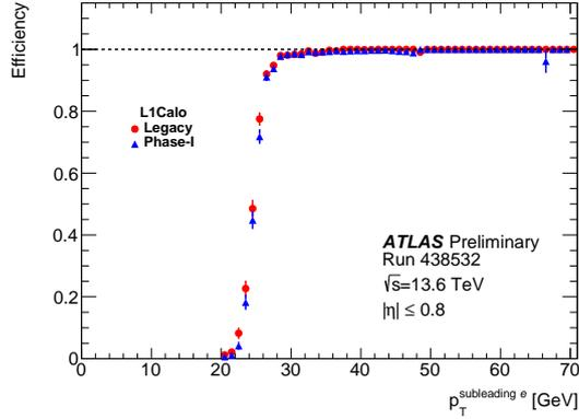
**Figure 1:** L1Calo single electron trigger efficiencies in the inner calorimeter barrel  $|\eta| < 0.8$ , measured using  $Z \rightarrow ee$  events with the tag-and-probe method, as a function of subleading electron  $p_T$ , for the Run 2 system (red) and for the Run 3 (eFEX-based) system (blue). Source: [2]
