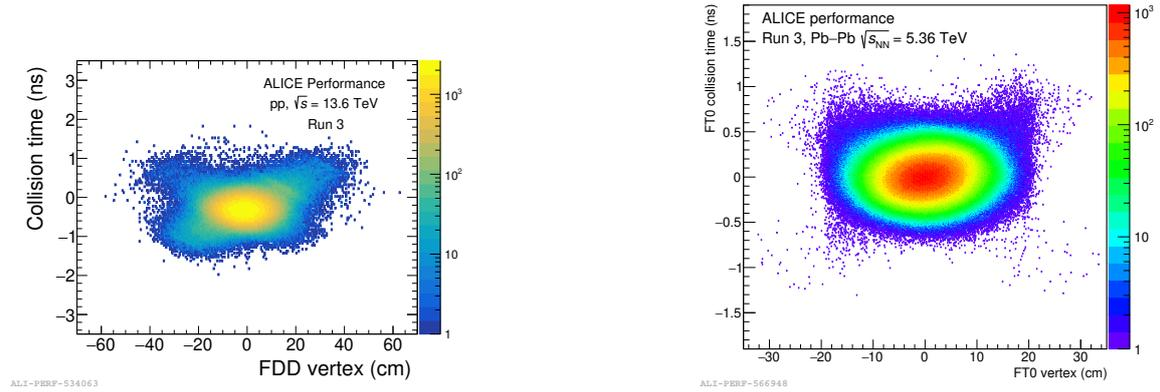
**Figure 3:** Correlation between collision time and vertex position as measured by FDD for pp collisions (left) and by FT0 for Pb-Pb collisions (right).
