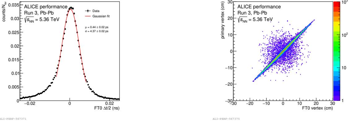
**Figure 2:** The FT0 time resolution (left), and the correlation between the FT0 vertex and the primary vertex (right).
