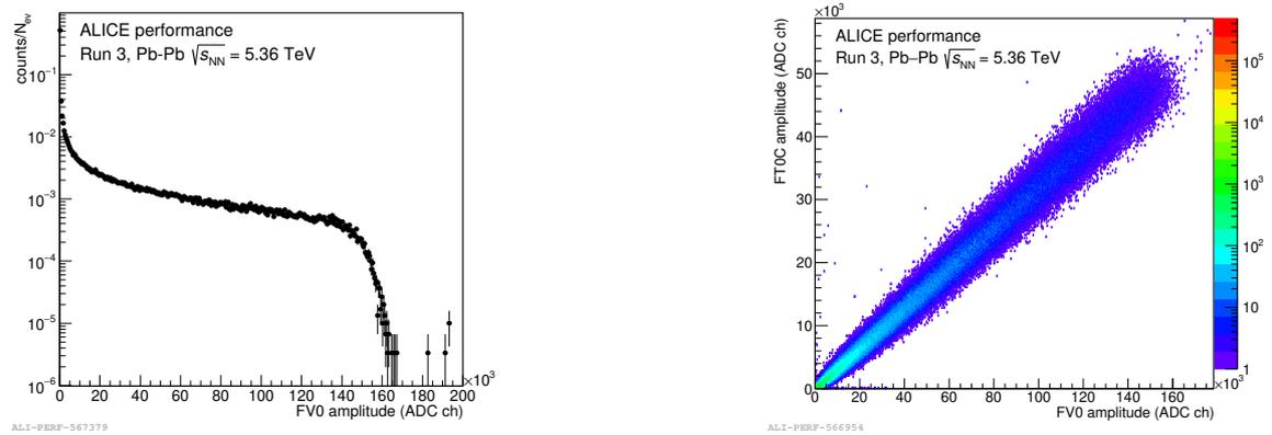
**Figure 4:** FV0 total charge distribution for Pb-Pb collisions (left) and correlation between the total charge of FT0-C and FV0 (right).
