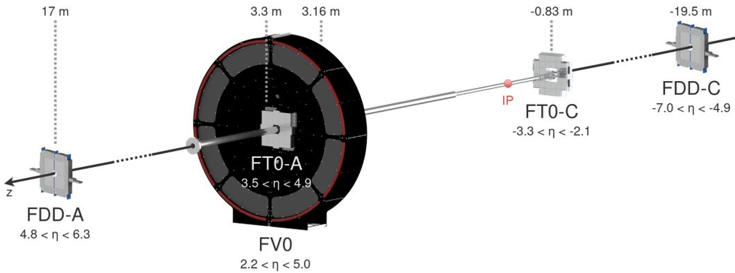
**Figure 1:** Schematic illustration of the FIT detector elements and their housing. The pseudo-rapidity coverage and distance from the interaction point of the detector elements are listed. For reference, the FV0 detector is about 1.5 m in diameter.
