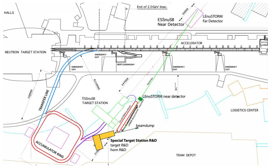
**Figure 5:** Implementation of the single target/horn target station (yellow), LEnuSTORM (racetrack storage ring in red), and LEMNB (instrumented tunnel in purple) in ESS site.
