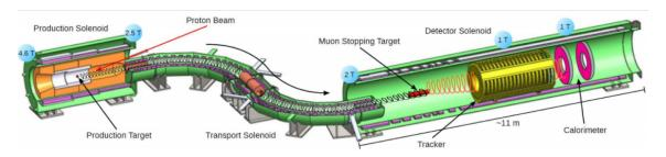
Figure 1: Schematic view of the Mu2e apparatus
