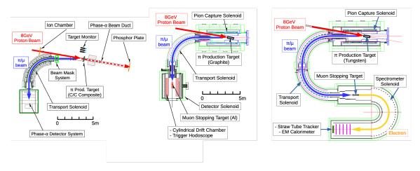
**Figure 6:** Three phases of the COMET experiment: Phase  $\alpha$  (left), Phase-I (center), and the proposed Phase-II (right).
