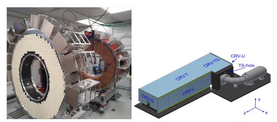
Figure 4: Left: Status of the construction of the calorimeter disks. Right: Sketch of the Cosmic Ray Veto.
