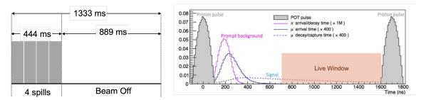
**Figure 2:** Left: 1.4 s structure of the main injector cycle and proton beam fraction delivered to Mu2e. Right: Mu2e pulsed proton beam structure.
