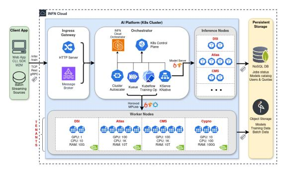
Figure 1: AI Platform: High-Level Architecture.
