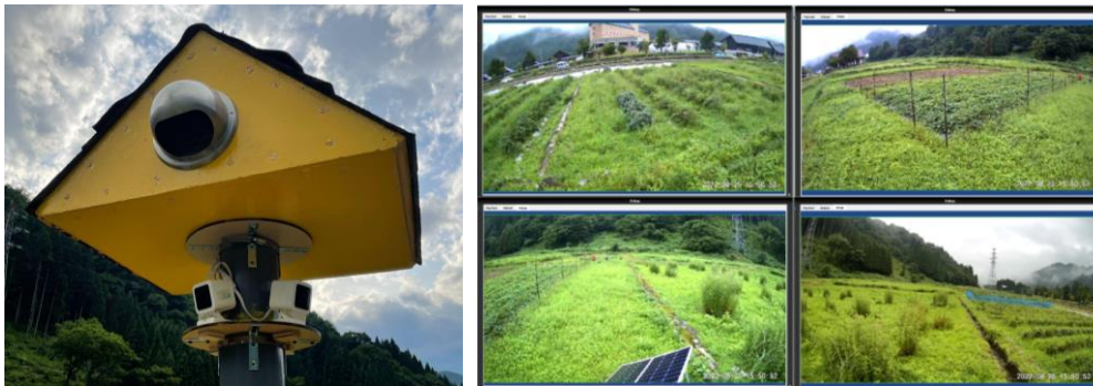
Figure 6: Four cameras are installed beneath the shutter (left) and Farmland Monitoring (right).
