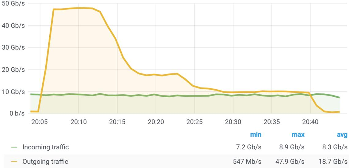
**Figure 2:** IHEP LHCONE traffic monitoring chart. The x-axis is time, y-axis is network bandwidth (Gb/s). The green and orange curves are IHEP LHCONE incoming and outgoing traffic, respectively. The min, max and avg are the minimum bandwidth, the maximum bandwidth and the average bandwidth within the time range depicted in the graph.
