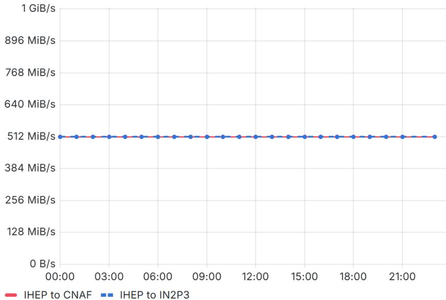
**Figure 9:** FTS Transfer Monitoring graph for IHEP to CNAF and IHEP to IN2P3 transfer directions at 512MiB/s bandwidth. The x-axis is time, y-axis is network bandwidth (MiB/s). The legends indicate transfer directions. In this test, we removed the direction from IHEP to JINR. The transfers from IHEP to IN2P3 and from IHEP to CNAF were smooth, the bandwidth reached 512MiB/s.
