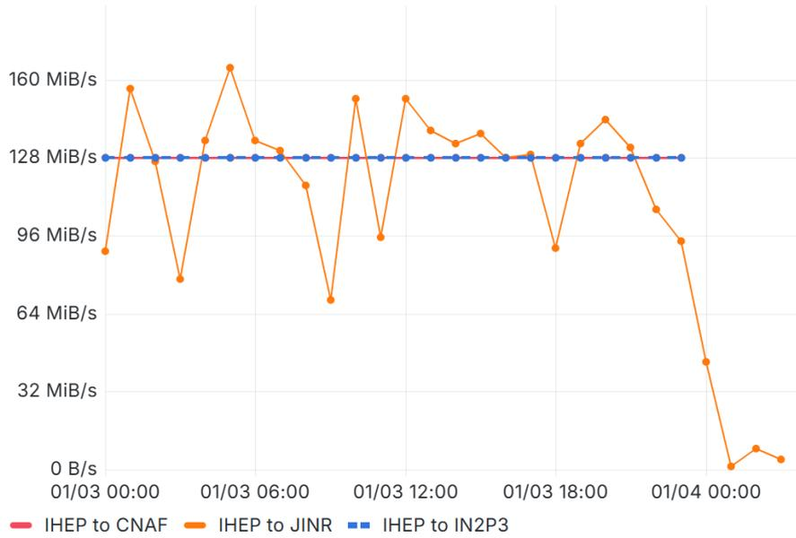
**Figure 6:** FTS Transfer Monitoring graph for three transfer directions at 128MiB/s bandwidth. The x-axis is time, y-axis is network bandwidth (MiB/s). The legends indicate transfer directions. The transfers from IHEP to CNAF and from IHEP to IN2P3 showed very good results, the bandwidth is consistently maintained at 128 MiB/s. The transfer from IHEP to JINR fluctuated significantly. This is because the network upgrade did not include the link between IHEP and JINR.
