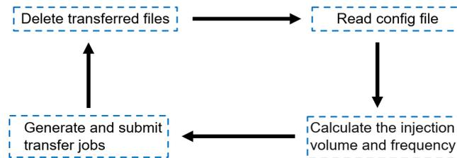
**Figure 3:** The flowchart of the data injection tool
