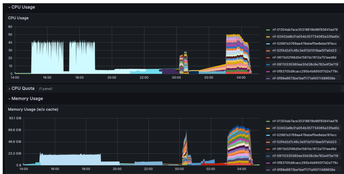
Figure 3: Resources used by the Whole Genomics Pipeline workflow, captured by Grafana. Each color/identifier represents a different pod, and thus, a different unit of work of the pipeline.
