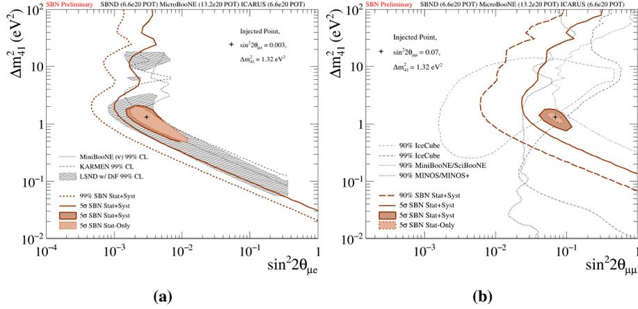
**Figure 2:** (a) Constraints on the  $\nu_e$  appearance and (b) on the  $\nu_\mu$  disappearance set by SBN at 99% (dashed line) and at  $5\sigma$  sensitivity (solid line) after 3 years of data taking.
