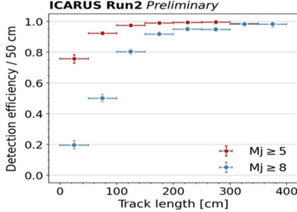
**Figure 3:** The trigger efficiency measured exploiting almost vertical cosmic muons independently selected by TPC tracks matched with CRT signals.
