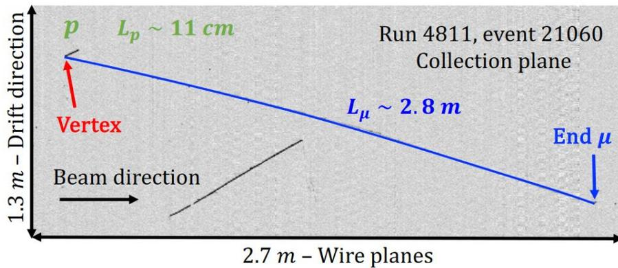
**Figure 7:** A BNB QE  $\nu_\mu$  CC candidate with 1 muon and 1 proton at the primary vertex found by the visual scanning procedure.
