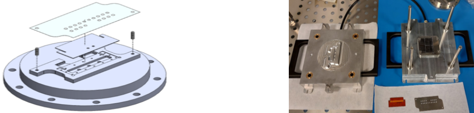
Figure 2: The figure shows the design (left) of the jigs and the actual tools used (left) to perform the module assembly at IFAE.
