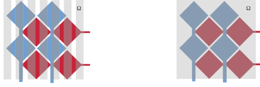
Figure 6: Diagram of the interconnected pad design, on the left prototype D3 with the strip resistive pattern on top of the readout, and on the right D4 with the full resistive layer.
