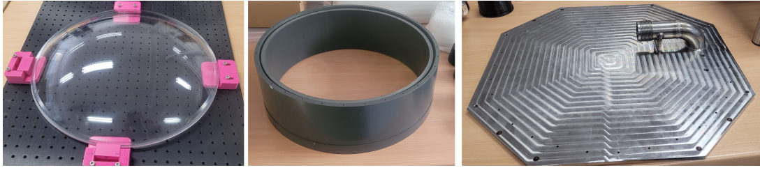
Figure 2: Mechanical Components of mPMT; Acrylic Dome, PVC cylinder and Back plate
