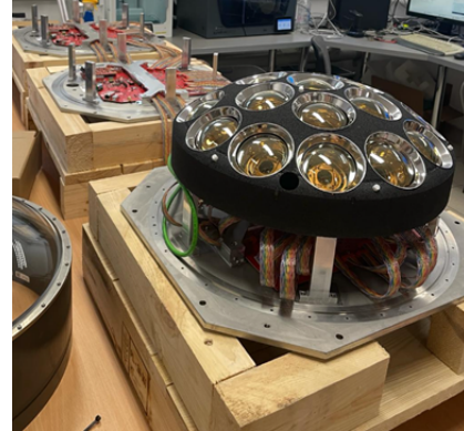
Figure 8: In-situ mPMT with PMTs and reflectors, ready to be gelled
