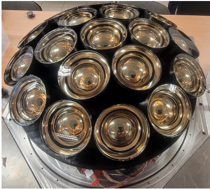
Figure 7: Ex-situ mPMT during assembly, with mounted gelled PMTs
