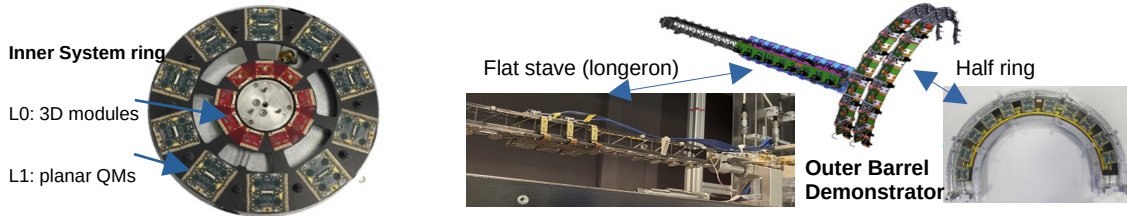
Figure 5: ITk-Pixel LLS prototype examples for IS ring and OB demonstrator.
