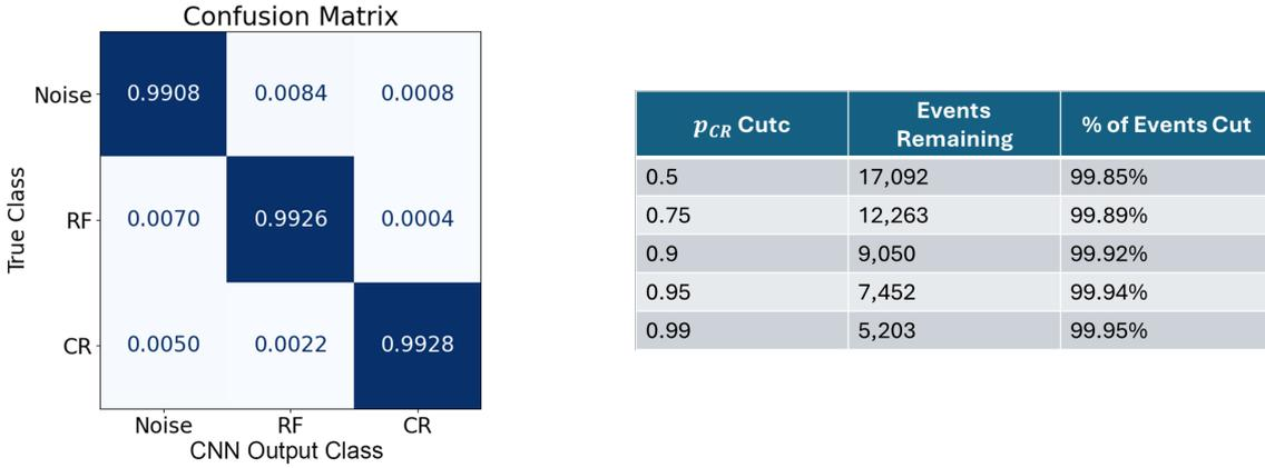
**Figure 3:** Performance of the classifier CNN trained to distinguish noise, cosmic ray, and other RF source waveforms. The left displays the confusion matrix which identifies how often the classifier labels a waveform correctly or incorrectly. The right displays the effectiveness of cuts for different thresholds of probability that a given event is classified as a cosmic ray.
