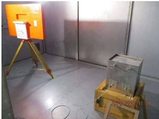
(a) Xbox inside RC with Antenna
