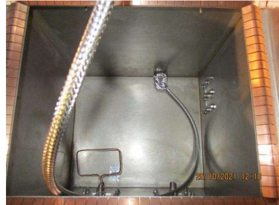
(b) Loop antenna on inside of Xbox
