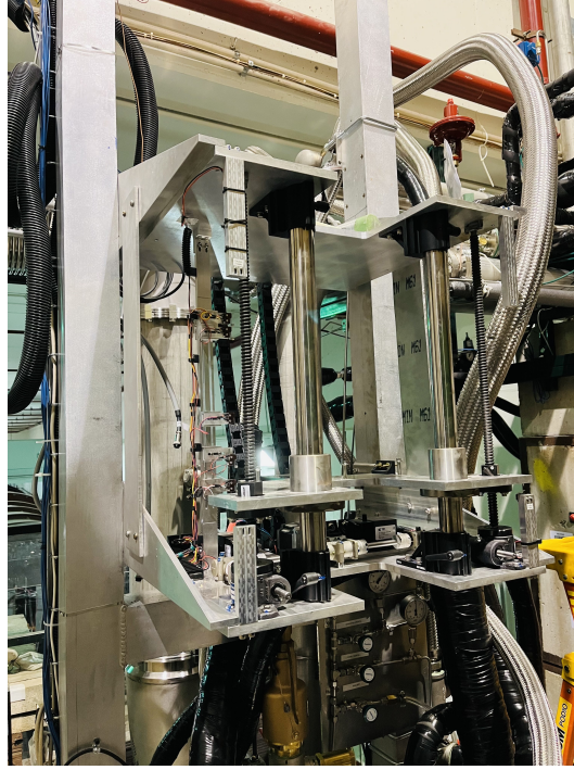
Figure 5: The target lifter system installed in the target cave
