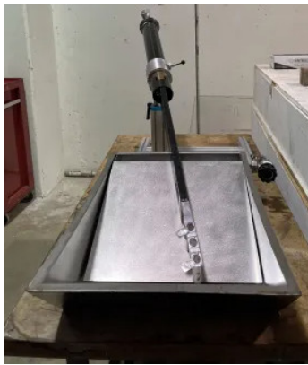
Figure 10: Stand and LN2 bath used to load target materials to target cells.
