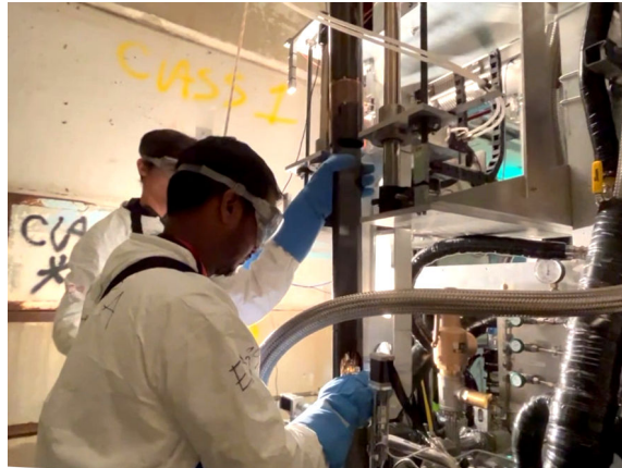
Figure 11: Scene of loading target material into the fridge.
