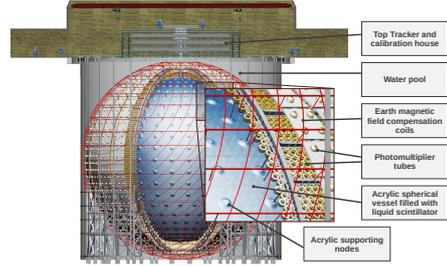
**Figure 2:** Schematic representation of the main JUNO detector [3].
