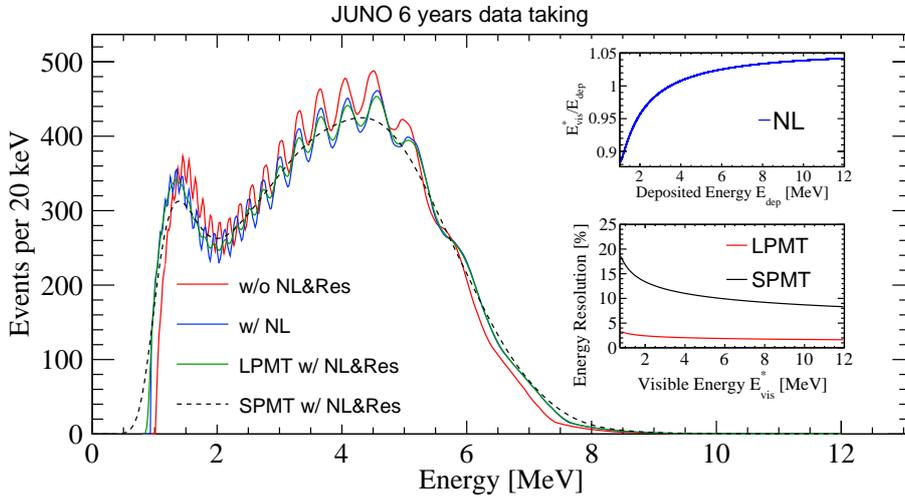
**Figure 3:** Expected prompt energy spectrum with and without the different detector response effects [10].
