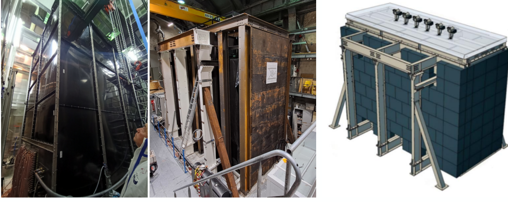
Figure 4: Left: photograph of the anti-Rn tent, middle: photograph of the incomplete iron shielding, right: drawing of the neutron shielding.
