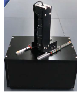
Figure 4: A new probe station for the quality check of the silicon pad sensors.
