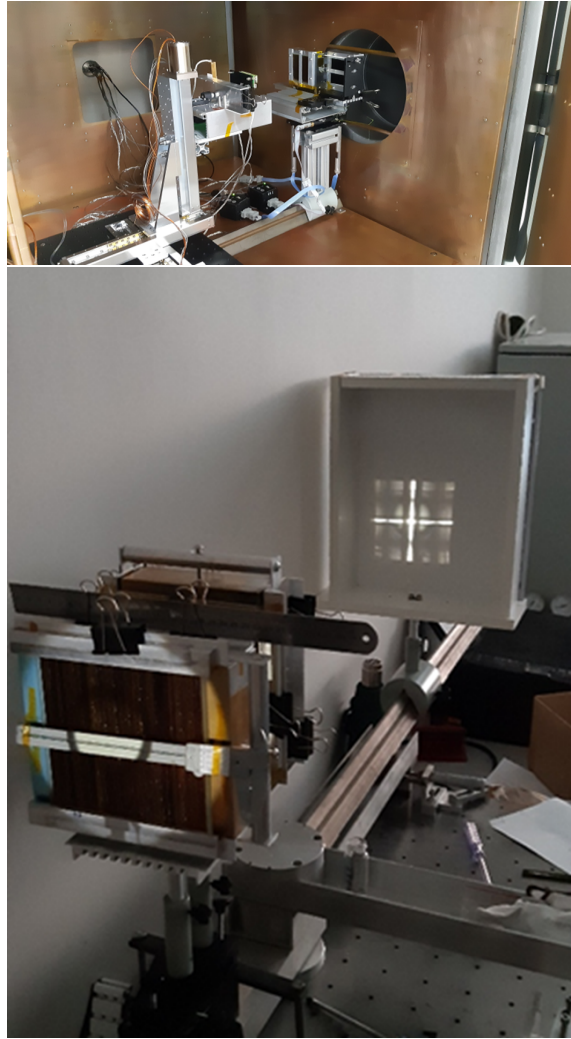
Figure 2: LE test modules at the X-ray test facility and in visible light tests. Photo courtesy RITE Prague.
