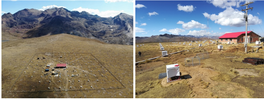
Figure 3: Photographs of the ALPACUITA array in Bolivia. In the left photograph, the mountain found in the back is Mt. Chacaltaya. The right photograph shows the ground view of the array. Each scintillating counter is protected by a water-proof white cover. The cables for signal and HV are connected to the central hut through the underground cable path.
