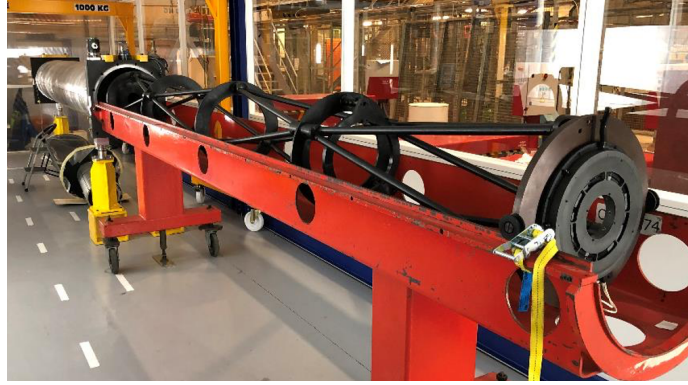
Figure 2: Picture of the CEDAR-H during construction at CERN. The black metal support frame for optical components is present to the right, including the diaphragm slit at the end. To the left, the silver cylindrical gas vessel is shown. [5]
