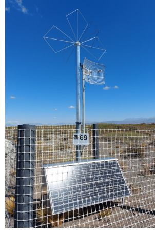
Figure 2: Image of one of the converted antennas at the G@A site. The 3-meter pole supports the antenna and the nut containing the LNA. Midway up the pole, the mesh communication antenna is installed. The space below the solar panel houses the battery, charge controller and front-end electronics. The entire setup is enclosed by a plastic fence.
