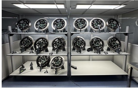
Figure 5: Production site at the Technical University of Munich. The picture shows the clean-room where the gel pads were produced, attached to the PMTs, and subsequently to the hemisphere glass.
