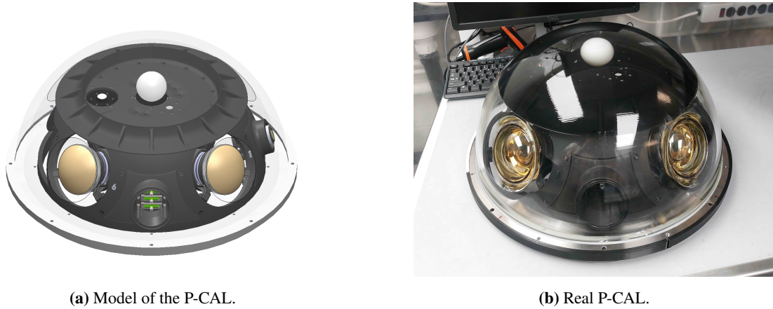
Figure 4: Model of the P-CAL module and picture of a P-CAL hemisphere with all the integrated components.
