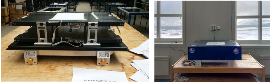
Figure 2: On the left, a close-up photo of one of the POLA-R muon detectors during assembly at CERN. On the right, the POLA-4 muon detector installed in the Gruvebadet Laboratory, at Ny-Ålesund
