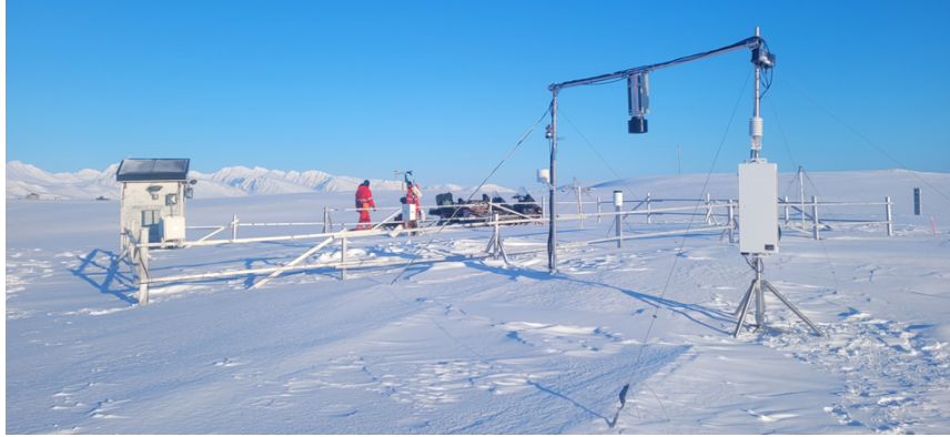
Figure 4: The cosmic-ray neutron sensors (CRNS) installed at the Bayelva site, near Ny-Ålesund
