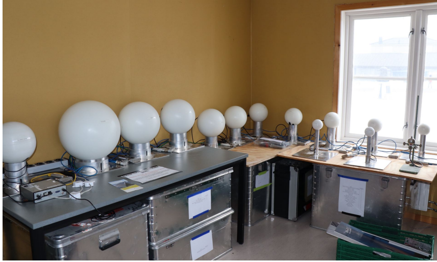
Figure 3: The Bonner Sphere Spectrometer (BSS) installed at Ny-Ålesund
