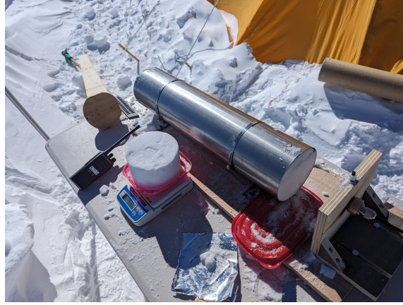
Figure 2: The core shaping rig: a metal cylinder of adjustable diameter used to trim the outer edges of firn cores to a consistent volume for gravimetric density measurements. The core is loaded into the rig from one side and pressed against a wooden board on the opposite side with a fixed gap. A 10 cm firn segment is shown being weighed on the tray below the apparatus.
