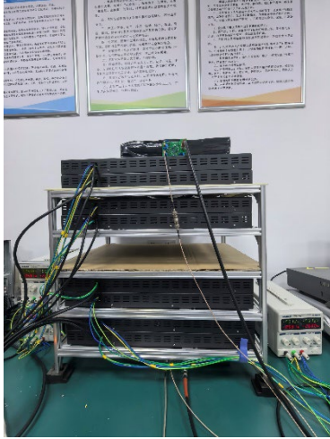
Fig.1 The Scintillating fiber detector
