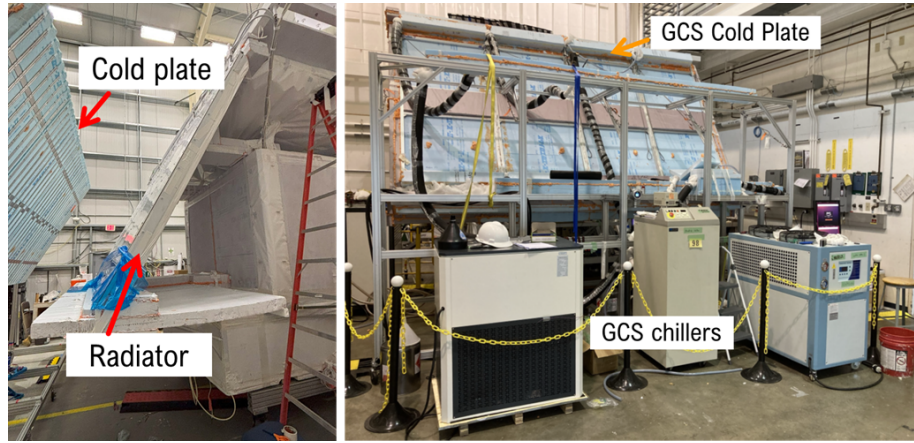
Figure 3: Photograph of the Ground Cooling System (GCS) setup. The system includes a commercial chiller, a cold plate attached to the radiator surface, and Styrofoam insulation to reduce environmental heat load.
