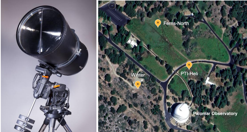
Figure 1: Left: Photograph of an individual PANOSSETI 0.5-m Fresnel telescope. Right: Planned locations of the first three telescopes at Palomar Observatory.
