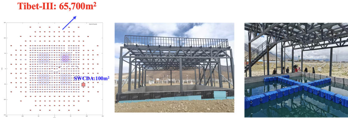
Figure 2: The prototype experiment of the SWCDA was completed at Yangbajing (4300 m). Left: The orange dots represent the Tibet-III array, the blue squares indicate the Tibet-MD detectors, and the orange square in the southeast corner of the array marks the location of the 100 m 2 SWCDA prototype detector. Center and Right: Physical photographs of the 100 m 2 SWCDA prototype detector.
