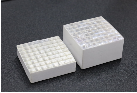
Figure 1: Pixelated GSO(Ce) scintillator. 13 mm thick (left) and 26 mm thick (right).
