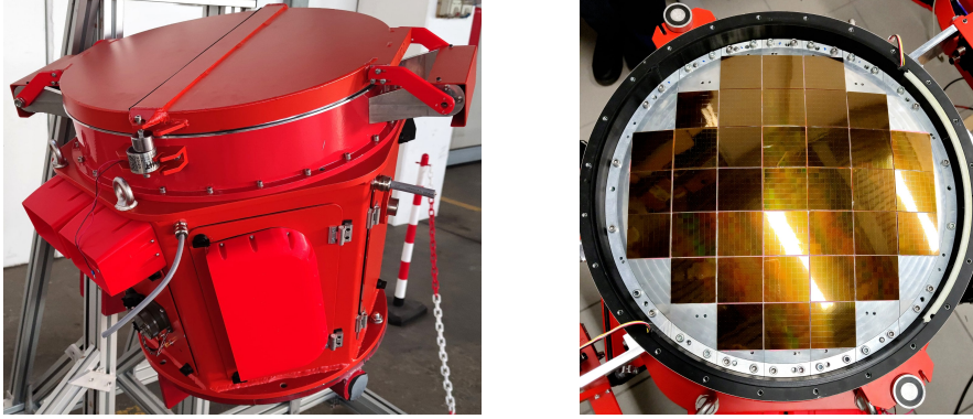
Figure 1: The ASTRI-1 Cherenkov camera during the assembly phase. Left) Camera body view with the lids closed. Right) Camera focal plane view with all the 37 PDMs mounted, SiPM tiles were still covered by a kapton protective film.
