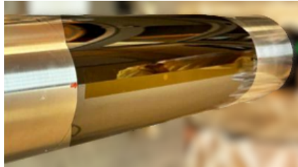
Figure 8: Initial engineering structure of two dummy silicon sensors connected and bent to a radius of 38 mm.
