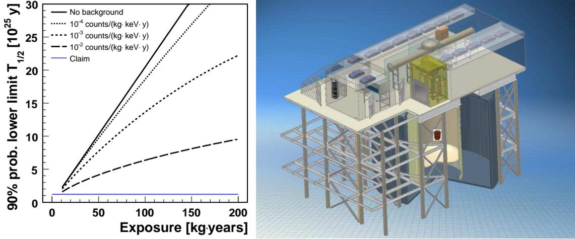
**Figure 1:** Left: Expected 90% probability lower limit on  $T_{1/2}^{0\nu\beta\beta}$  as a function of exposure for different background indices (taken from [6]). Right: Schematic view of the GERDA setup. The detector array is sitting in the center of the cryostat. The cryo tank is surrounded by a water buffer serving as additional shield and as a muon-Čerenkov veto system. The detector array is loaded through a lock system located in a clean-room on the top of the tank.
