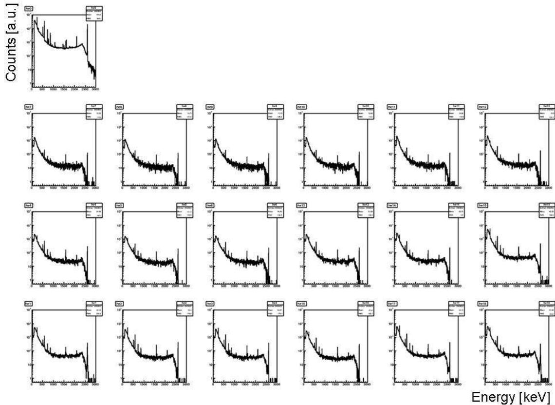
**Figure 4:** Calibration spectra of the core and all 18 segments of the segmented n-type HPGe detector operated in liquid nitrogen taken with a  $^{228}\text{Th}$  source.
