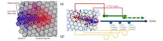
**Figure 5:** Example for a slowly-developing image of a 15 TeV shower. Colour coding is from red (early) to blue (late), with a total image duration of 55 ns. The colours of the clusters (hexagons) indicate the local triggering and readout times in the case of sliding readout
