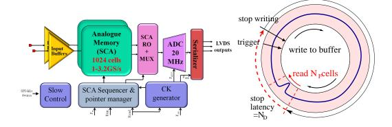
**Figure 2:** Left: Diagramme showing the functional elements of the NECTAr chip. Right: Cartoon sketch of the analogue ring buffer.
