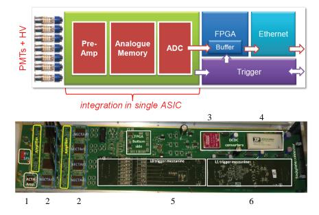
**Figure 3:** A NECTAr prototype board including ACTA amplifiers (1), NECTAr0 chips (2), ALTERA FPGA (3), DC/DC converters (4), L0 (5) and L1 (6) trigger mezzanine boards.
