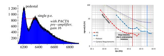
**Figure 4:** Prototype results. Left: amplitude distribution measured with a weakly-illuminated PMT, using a PACTA pre-amplifier. Right: charge resolution as function of the input amplitude, for the high-gain and low-gain channels, compared to CTA specifications.
