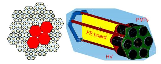
**Figure 1:** Left: Section of a camera made up of 7-pixel clusters. Highlighted is a possible combination of adjacent clusters used for triggering. Right: sketch of a 7-pixel cluster showing its main components.
