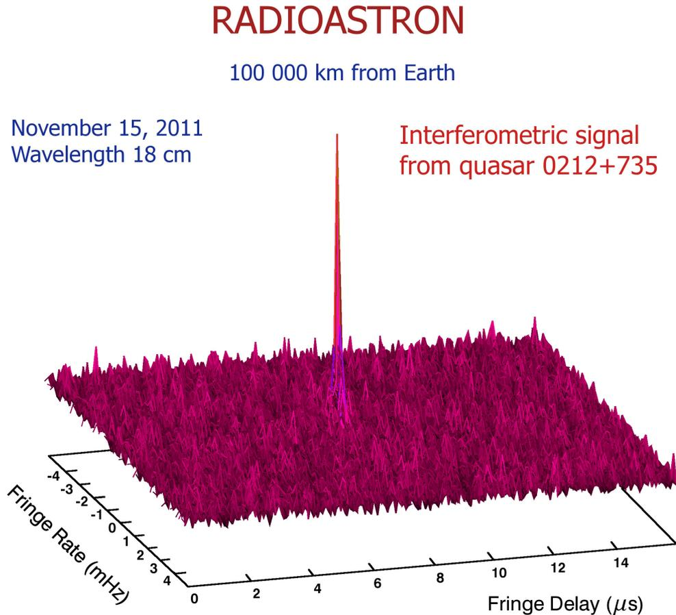
**Figure 2:** The first fringes found by the Space-VLB interferometer RadioAstron. Interference signal from the quasar 0212+735 on a 8,100 km projected baseline between RadioAstron and the 100-m MPIfR radio telescope near Effelsberg, Germany, observed on November 15, 2012. The wavelength of the observations was 18 cm. The plot shows the fringe amplitude versus residual delay and residual fringe rate in a single 16 MHz wide channel.
