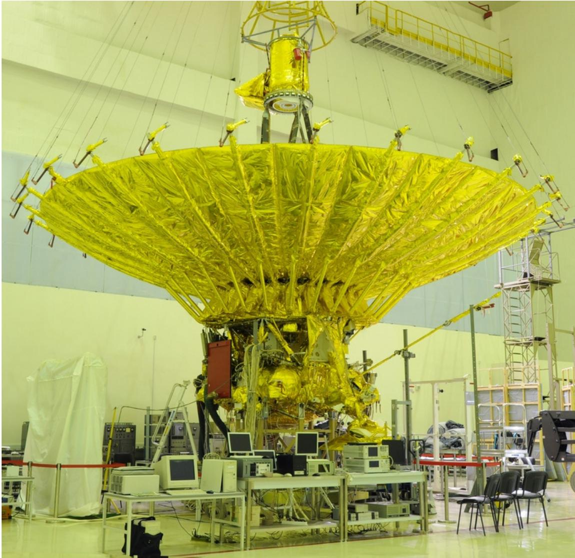
**Figure 1:** The space radio telescope Spectrum-R undergoing tests in Lavochkin Association.
