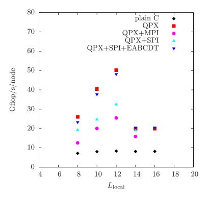
**Figure 1:** Single BG/Q node double precision performance of the hopping matrix in Gflop/s as a function of  $L_{local}$ . "Plain C" and "QPX" correspond to measurements with communication switched off using a plain C implementation and one including QPX instructions, respectively. The other points include communication, see text for details.
