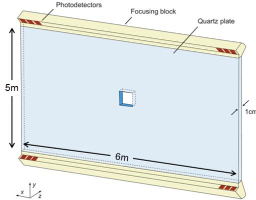
**Figure 1:** The TORCH detector design. Particles pass through the quartz plate producing Cherenkov radiation which is reflected to the photodetectors via focussing optics. Dimensions shown are for the TORCH detector located 9.5 m from the interaction point of LHCb.
