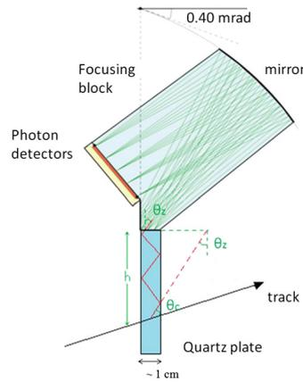
**Figure 4:** A cross section of the TORCH optical design. The angle  $\theta_z$  is mapped by a mirror onto a position on the photodetector surface.
