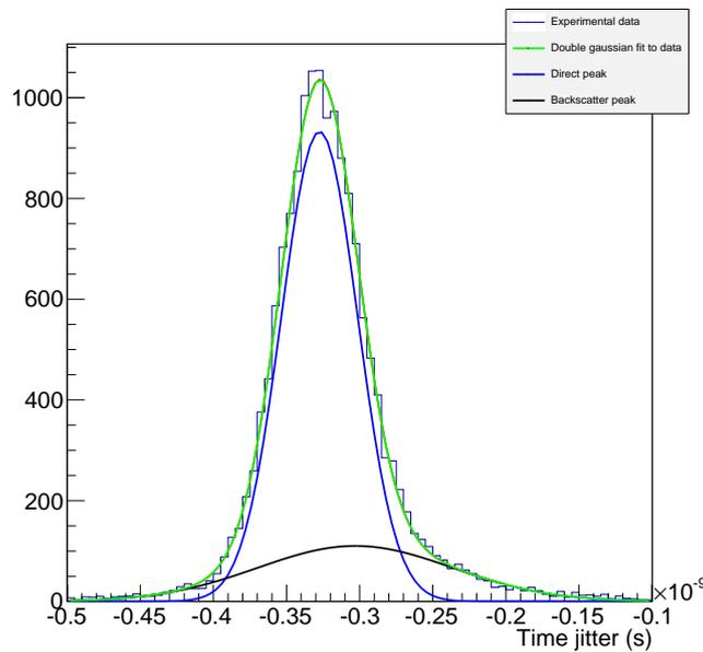
**Figure 6:** Timing distribution for the phase 1 MCP-PMT showing the time of arrival of the signal relative to the laser trigger. The distribution shown is inclusive of detector resolution, trigger jitter and the timing spread of the laser pulse.
