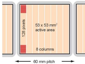
**Figure 3:** Schematic of the required TORCH MCP-PMT granularity and pitch [2]. Options regarding implementation are in progress.
