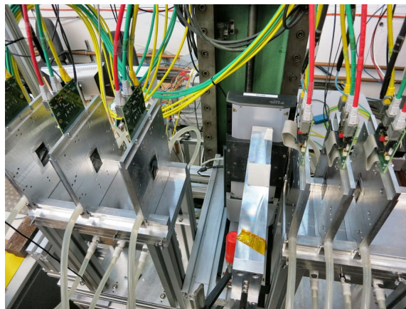
Figure 1: The EUDET/AIDA telescope consisting of two arms each equipped with three MIMOSA26 planes, and in-between a device of the CLICpix collaboration as device-under-test. Courtesy D. Dannheim.
