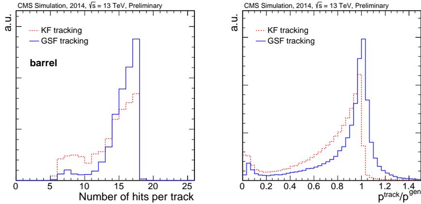
**Figure 2:** Number of reconstructed hits per track in the barrel (left) and ratio between the reconstructed track momentum and the generated one (right) for electrons tracks at HLT. Distributions are shown for tracks reconstructed with the Gaussian Sum Filter and the Kalman Filter. Similar selection as in Figure 1.
