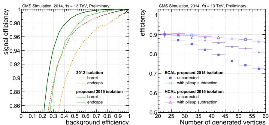
**Figure 3:** (Left) Performance curves of pileup-corrected electron isolation at HLT, comparing the detector based setup used in Run I to the simplified PF-based method. (Right) Signal efficiency of the latter method in the barrel, with and without pileup subtraction, with working points adapted for illustration purposes. The signal selection is similar to Figure 1, while background objects are triggered from a QCD sample.
