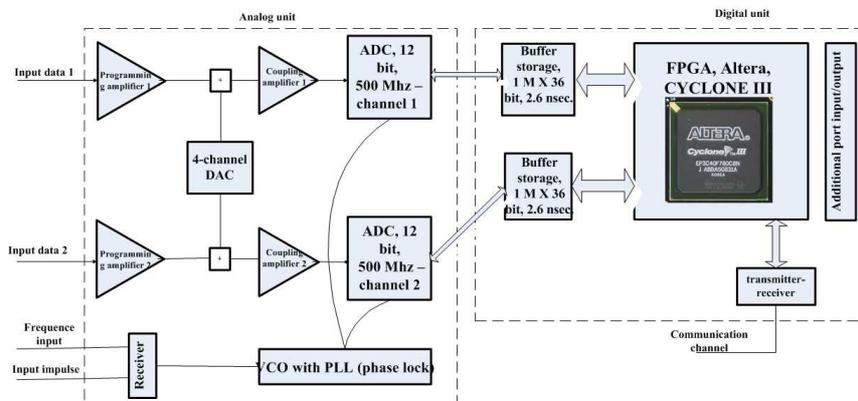
**Figure 2:** Functional circuit of data acquisition system
