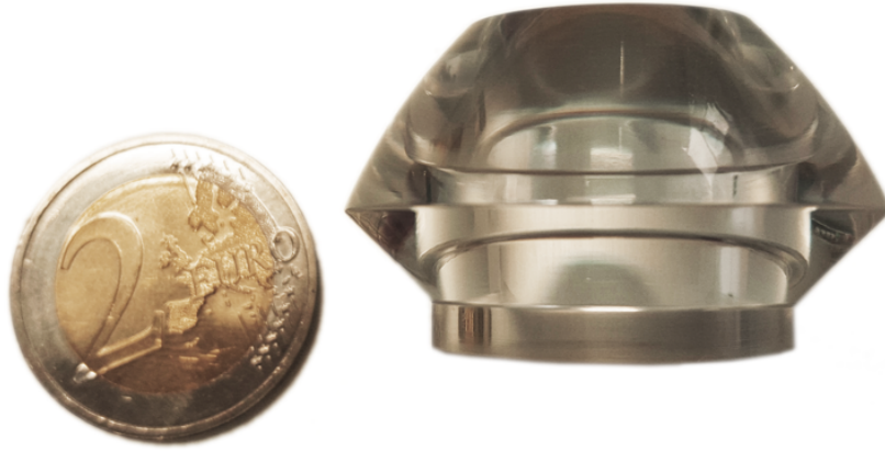
Figure 3: Photograph of the light concentrator which is part of the target head in the “mirror” design. The length of the concentrator is \Delta h = 20 mm. The neighboring coin sets the scale.
