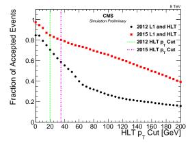
**Figure 3:** Fraction of simulated signal events passing the special-purpose trigger with respect to the generator level, as a function of the HLT  $p_T$  requirement, for the trigger configuration in 2012 (black) and the configuration to be used in 2015 (red). The simulated signal is the production of long-lived leptons (q = 2e, m = 500 GeV) stopping in the detector (typically a few meters from the interaction point) and decaying to 2 back-to-back muons.
