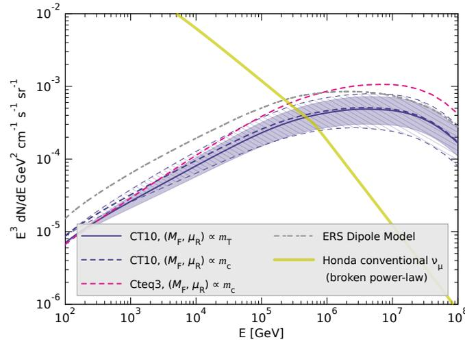
**Figure 4:** Prompt neutrino flux as a function of the neutrino energy together with the conventional component (yellow curve). The uncertainties are due to the renormalization and factorization scale variations in the calculation. Parton distribution function uncertainties are not included in the plot.
